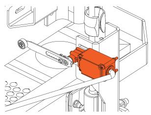
Figure 24: Platform position switch
