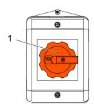
Figure 12: Bottom platform control box, automatic send configuration for fences with trapped key or electrical switch monitoring system
