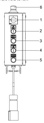
Figure 13: Bottom platform control box, send/call configuration
