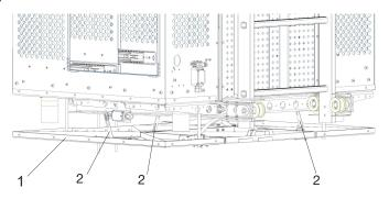
Figure 20: Bottom obstruction device
