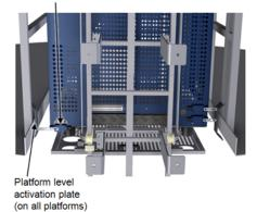
Figure 5: Platform level switch
