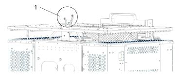
Figure 19: Top limit and Emergency top limit switches
