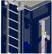
Internal manual release of guard locking
