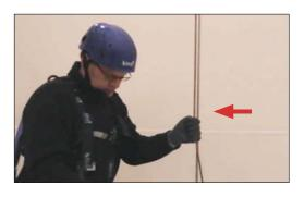
**Step 4 –** The BlocStop should lock onto the safety wire. Technician 2 checks so and reset the BlocStop again by pulling downward on the reset lever.
