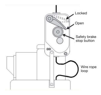
**Step 2 –** Person wearing appropriate PPE climbs roughly 1/4 of the way through the upper hatch so they can reach the drive cable. With a gloved hand, reach above the BlocStop and push the excess wire down so that a loop of wire is moved between the BlocStop and the motor.
