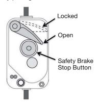
**Step 5 -** Repeat steps 3 and 4 for a total of 3 tests. If the unit does not pass all 3 tests, the unit must be locked out for repair. If the unit passes all 3 tests, go to step 6.
