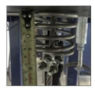
**NOTE** - If the safety cable does not appear to have enough travel to perform the rapid pull, adjust the spring below the deck so that the spring has an approximate resting state length of 2.5". This will only need to be done once per tower, if at all. Refer to the Avanti User's and Installation Manual page 57.
